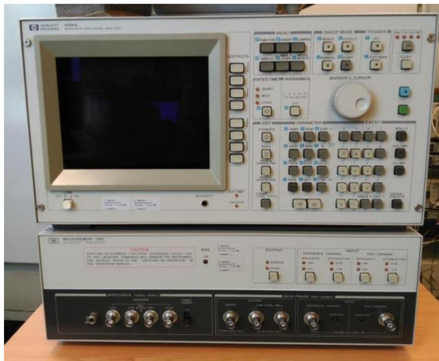
Figura 27. HP 4194A Impedance/Gain-phase analyzer
