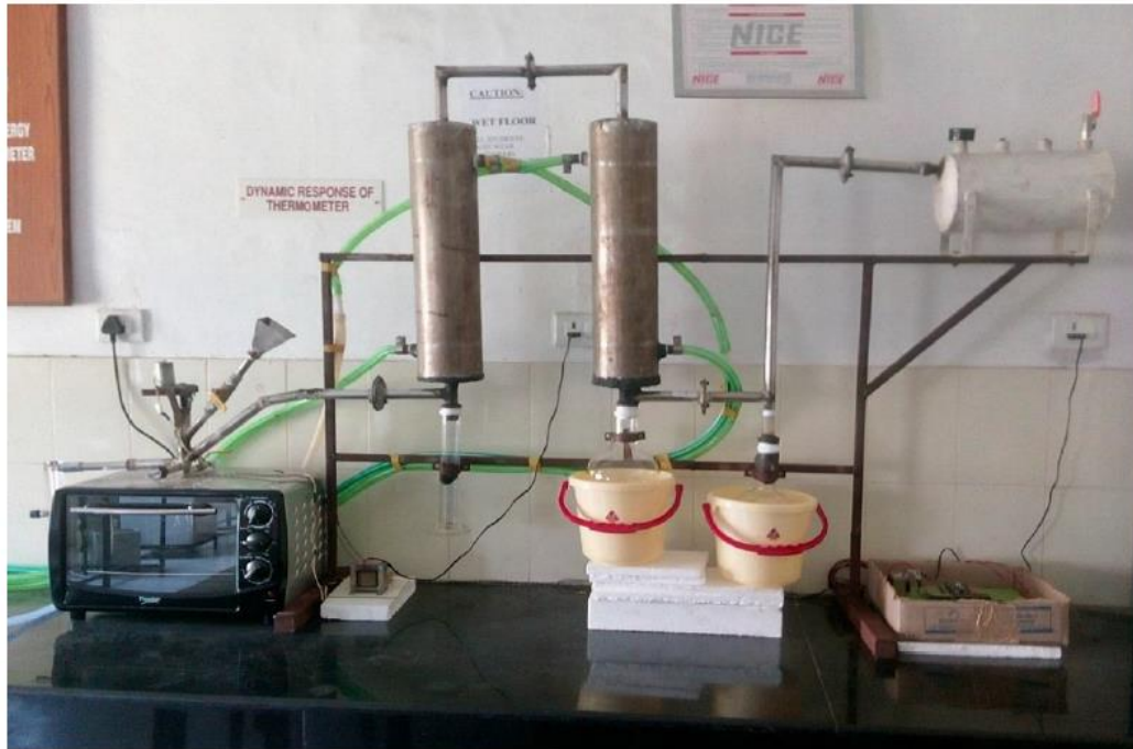
Figure 32: Experimental setup of the microwave assisted pyrolysis procedure (Aishwarya, 2016).
