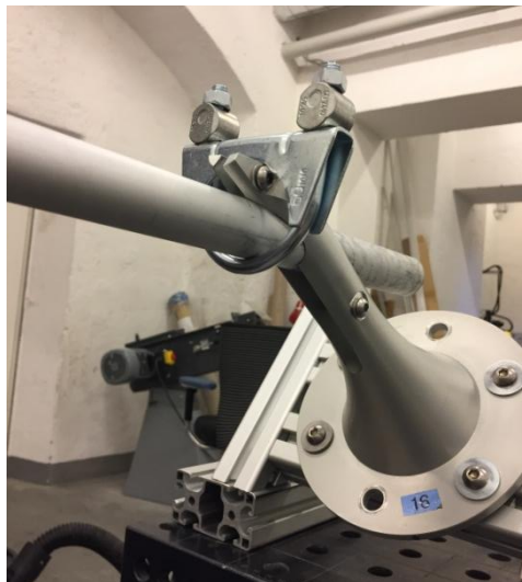
Figure 36. Improved fixation of the cane to the clamp
