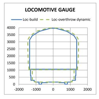
FIGURE 5. BUILT/DYNAMIC LOCOMOTIVE GAUGE
