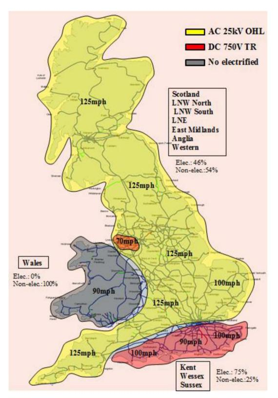
Figure 6. Overview in electrification systems and maximum primary operation speeds in  $\mbox{P/S}$  routes
