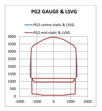
FIGURE 4 CENTRE/END STATIC GAUGE PG2 AND LSVG
