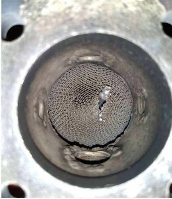
Figure 44 Damages in the pre-catalytic converter due to the high temperatures
