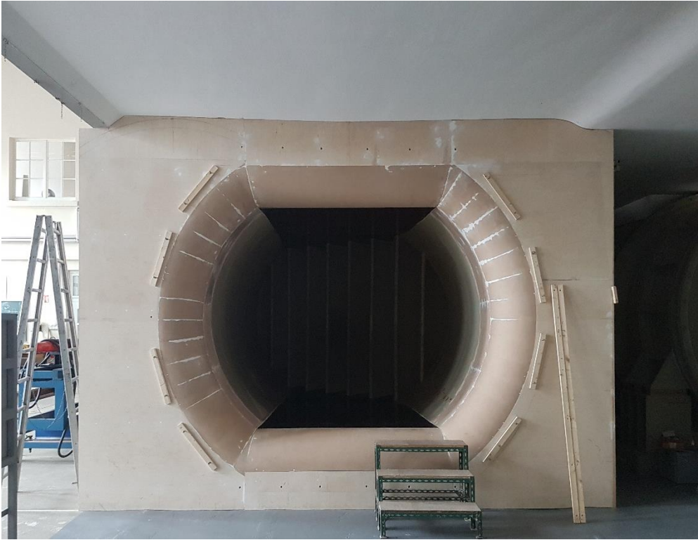
Figure 19. New wind tunnel diffuser [6].
