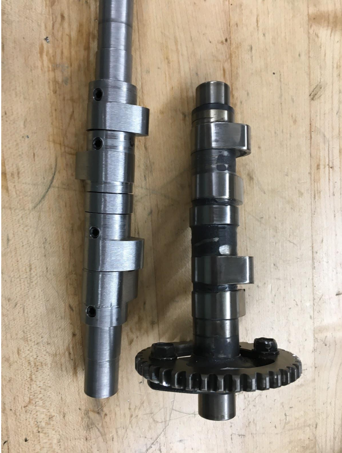
Figure 37: Cam Assembly (Left) and Stock Camshaft Photograph
