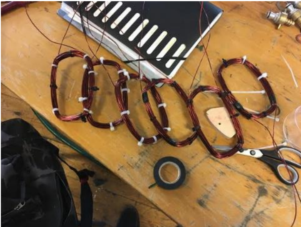
Figure 39- Coils manufacture for the three phase Radial generator
