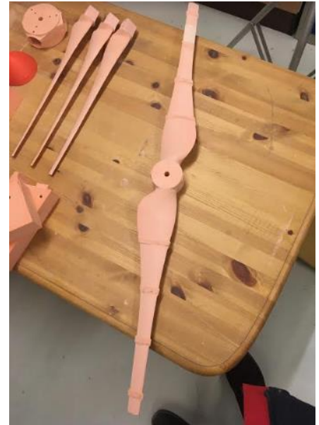
Figure 38- Turbine before the polishing process
