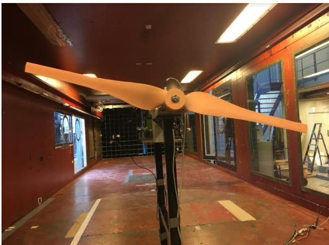
Figure 43- Rotor assembly in the wind tunnel
