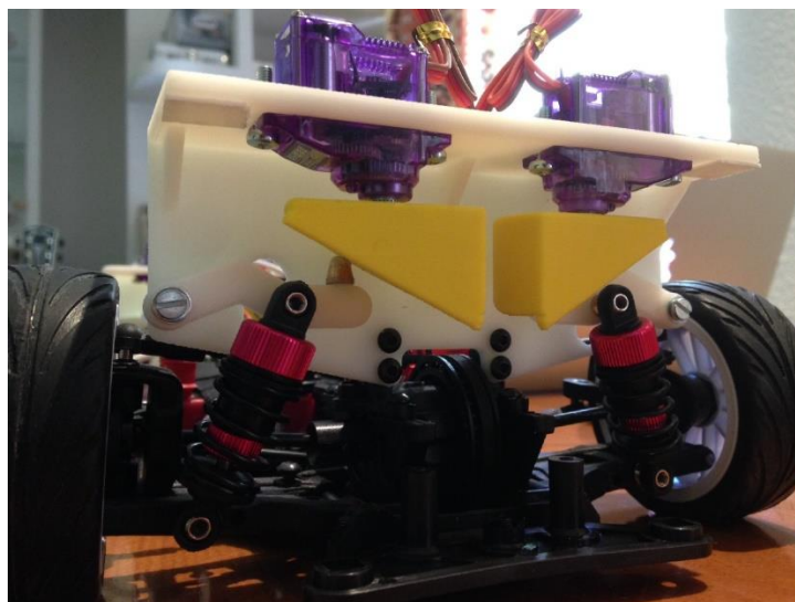
Figure 2.3.: Active suspension system installed on the Prototype.
