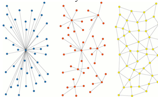
Figure 5 Network topologies: centralized, decentralized, distributed
