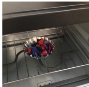
Figure 7: mould with plastic pieces into the electric oven.
