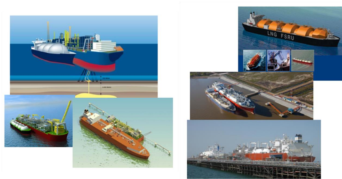
Picture 15: Floating Storage and Regasification Units – FSRU (Gas Natural Fenosa Materials, 2015)
