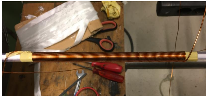
Figure 74: Winding process of the solenoids
