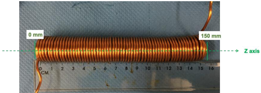
Figure 77: Solenoid 2 mm. 3 layers. 15 cm
