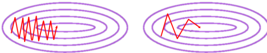
Figure 2.33. Optimization algorithms with (right) and without (left) a momentum term.
