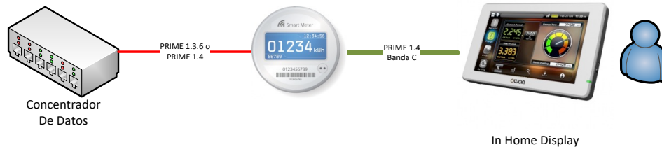
Figure 7. Configuration from the communication between the meter and the In-Home Display [13]
