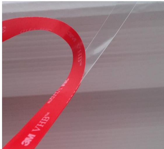
Figure 1 – VHB double sided adhesive foam [21]
