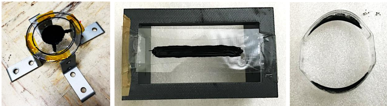
Figure 8 – Configurations of dielectric elastomer actuators
