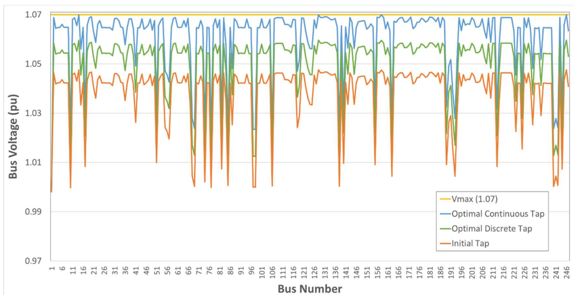
Figure 5.4: Peak hour (20:00h) voltage profile depending on tap position
