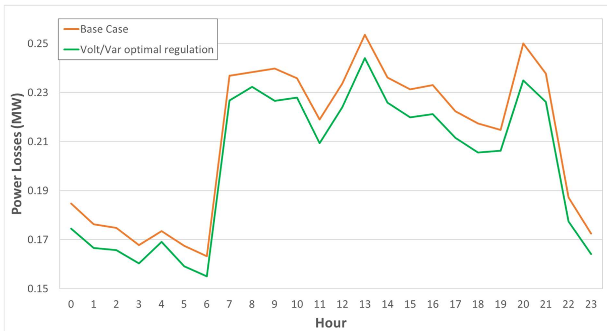
Figure 5.20: Power losses reduction with Volt/VAr regulation
