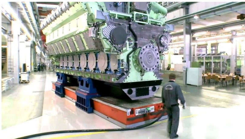
Figura 2-11. Motor Sulzer 12RTA96C. Fuente: https://www.youtube.com/watch?v=VcSMwRgRDV8
