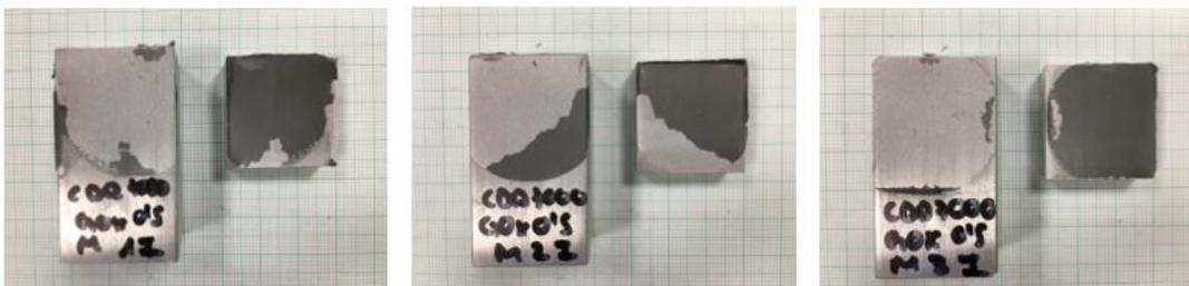
Fig. 51: Probetas Charpy GNPox 0.5% M
