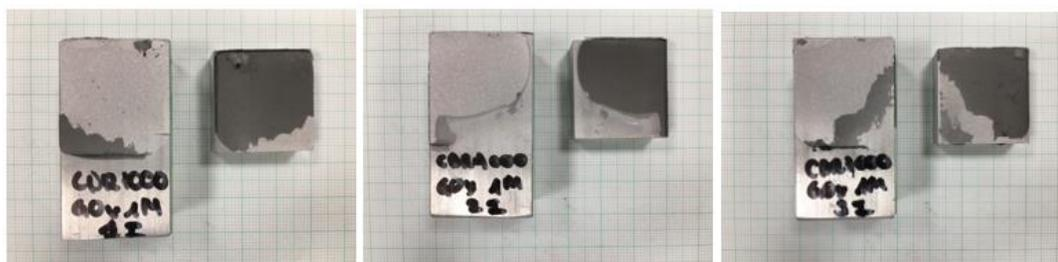
Fig. 52: Probetas Charpy GNPox 1.0% M
