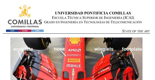
main plane Figure 29: Front Wing Parts
