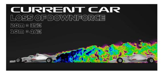
Figure 3: Loss of downforce following a 2021 F1 car
