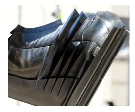
Figure 26: Strakes in Front Wing
