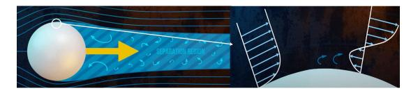
Figure 35: Flow separation
