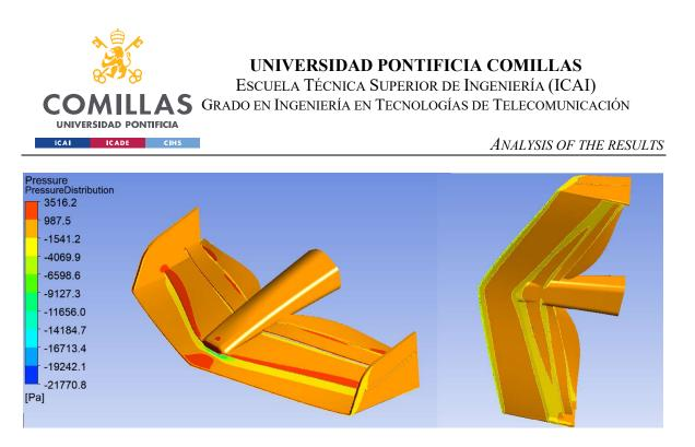
Figure 51: AMR22 Frontwing Pressure Distribution
