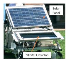
This NESMD solution is still under development since the membrane is manufactured in the laboratory as it is not available on the market. Unlike other distillation systems, this one has a solar panel that provides the extra energy needed to reach the boiling point of the water. Finally, it should be noted that this system is capable of producing a flow rate of 0.75 l/(m2\*h) which makes it less productive than other standard solutions on the market.
