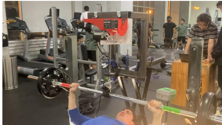
Figure 44: Bench Press Smart Helper in Real Gym Test
