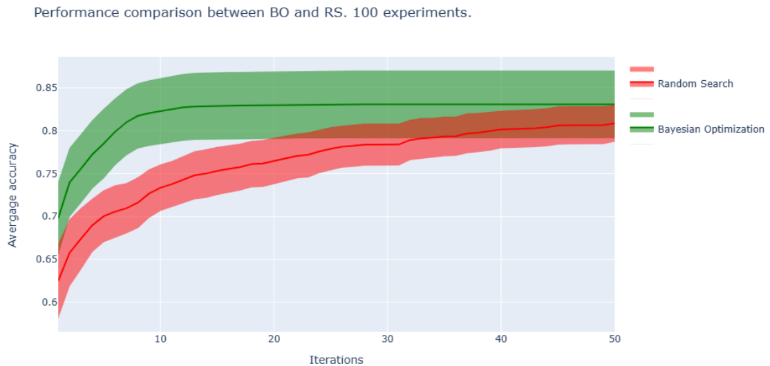
Picture 7: Comparison of the results obtained by the Bayesian model and Random Search for 100 experiments of 50 iterations
