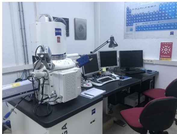
Figure 6. Zeiss Auriga Gemini Scanning Electron Microscope used for fractographic and compositional analysis
