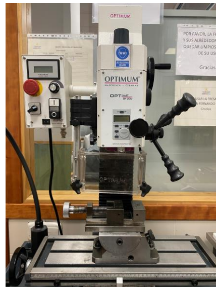
Figure 3. Micromet cutting tool (left) and Optimum milling machine (right) used for coupons fabrication.
