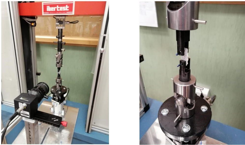
Figure 5. Testing setup (camera and tensile test machine, left picture) and clamping system (right picture) used for tensile tests.
