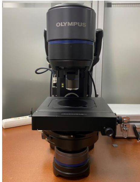
Figure 4. High-resolution Olympus digital microscope used for performing preliminary imaging.
