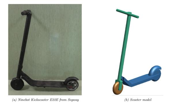
Figure 1: Scooter used and model
