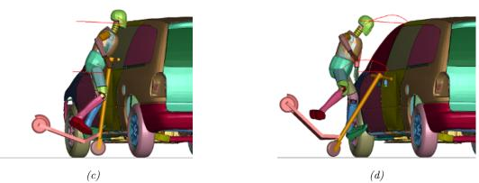
Figure 3: Kinematics with Dummy Hybrid III  $50^{th}$  without helmet
