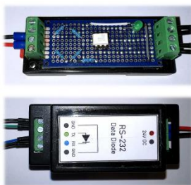
FIGURE 22. Data diode. The data diode is assembled using a PCB (Printed Circuit Board) and a specially adapted plastic case designed to be mounted on DIN rails. This feature is particularly significant as it enables the data diode to be conveniently installed alongside the IoT gateway.
