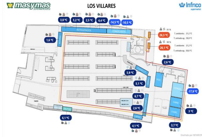
FIGURE 1. The installation has 6 refrigeration units, 2 freezers, 4 refrigerated display cabinets and four storage chambers (3 refrigerated and 1 freezer). Source: Kiconex.
