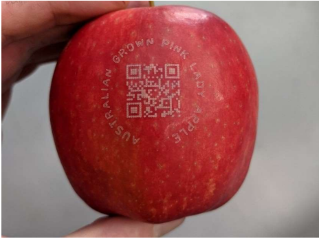
FIGURE 4. APPLE WITH LASER ENGRAVED QR [8]
