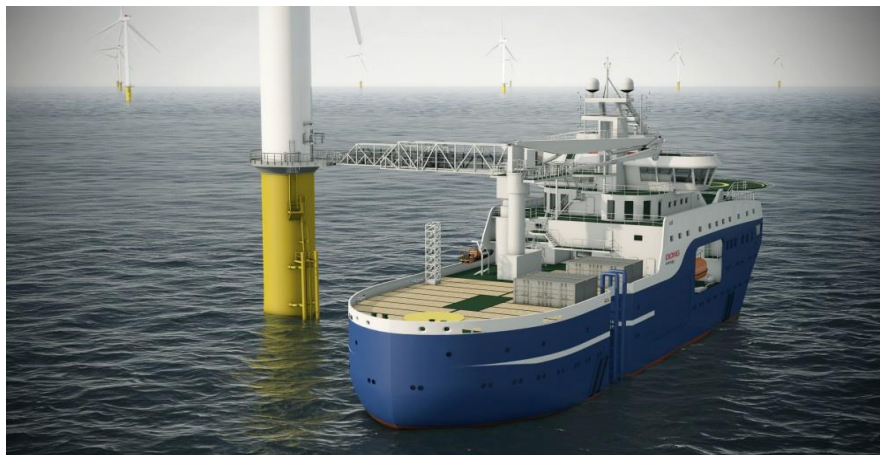
Figure 1: eco-SOV vessel accessing an offshore wind farm.
