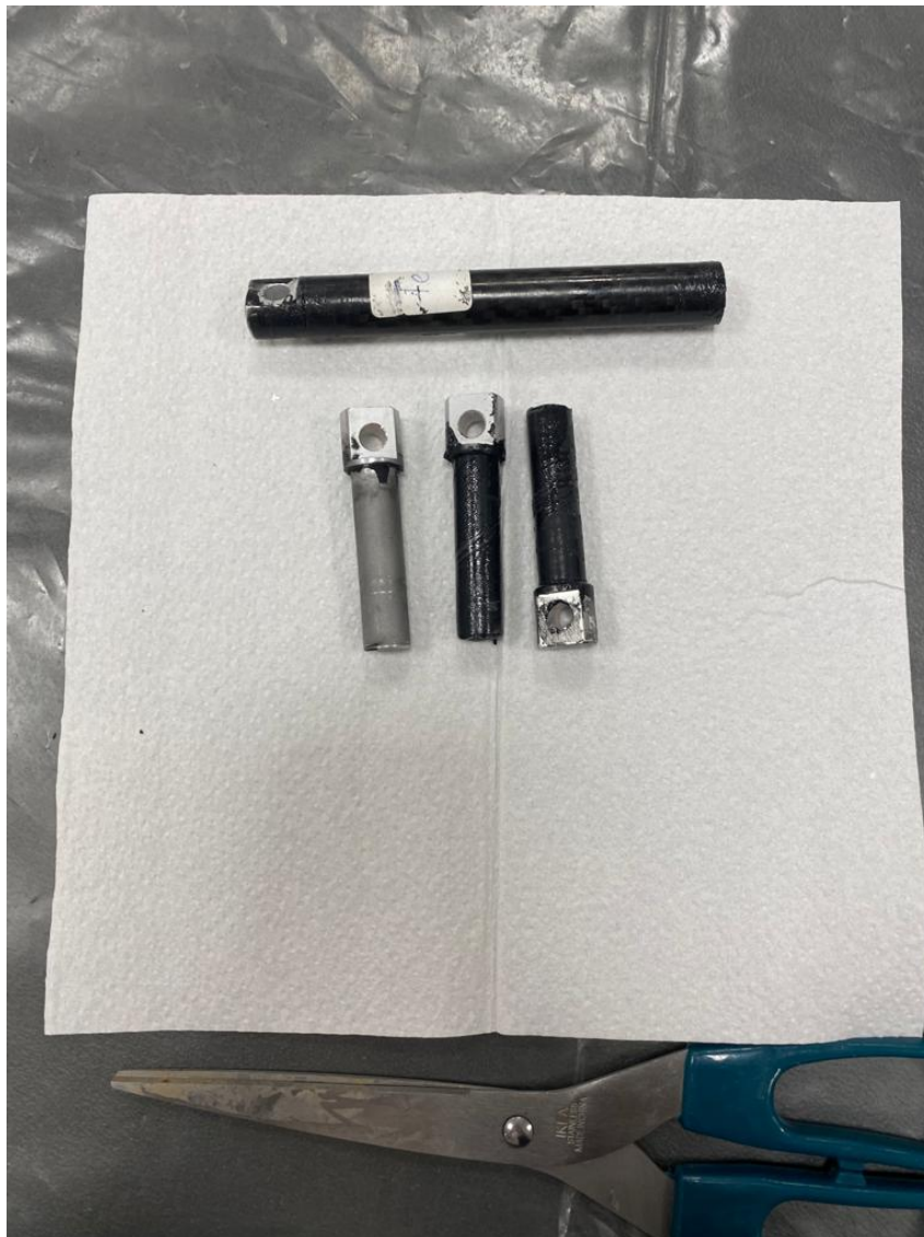
Figure 26: suspension test bar after failure
