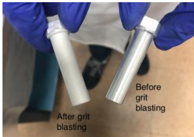
Figure 20: surface treatment for inserts
