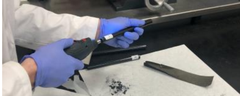
Figure 21: surface preparation carbon tubes
